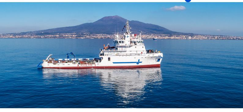
The Urbano Monti multi-purpose vessel is designed to carry out various services for the offshore industry. The ship built in 2007 has been equipped with the highest standards demanded of a modern internationally operating multi-purpose survey vessel: multi-beams echo sounder, side scan sonar, sub bottom profiler, magnetometer and ultra short base line.
